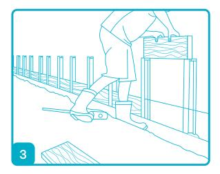
Cut timber rails to length before slotting them into the SureWall retaining posts. Prior to back filling, suitable drainage is recommended, i.e. slotted drainage pipe with FilterSleeve® laid in a trench of drainage metal, additionally the drainage metal can be wrapped in a DuraForce® or FilterPlus® geotextile.
